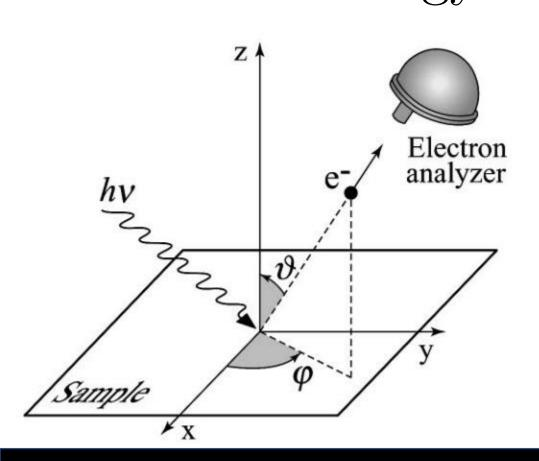
2D sample Electron momentum constrained to an x-y plane so momentum
