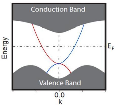
These systems contain non degenerate spin states which are crucial for utilization in spintronics
