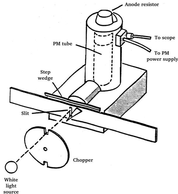
Figure 1.3: Experimental arrangement for measuring the linearity of the PM
