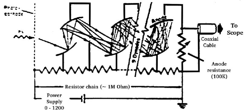
Figure 1.2: Schematic of the RCA 931 Photomultiplier Tube.
