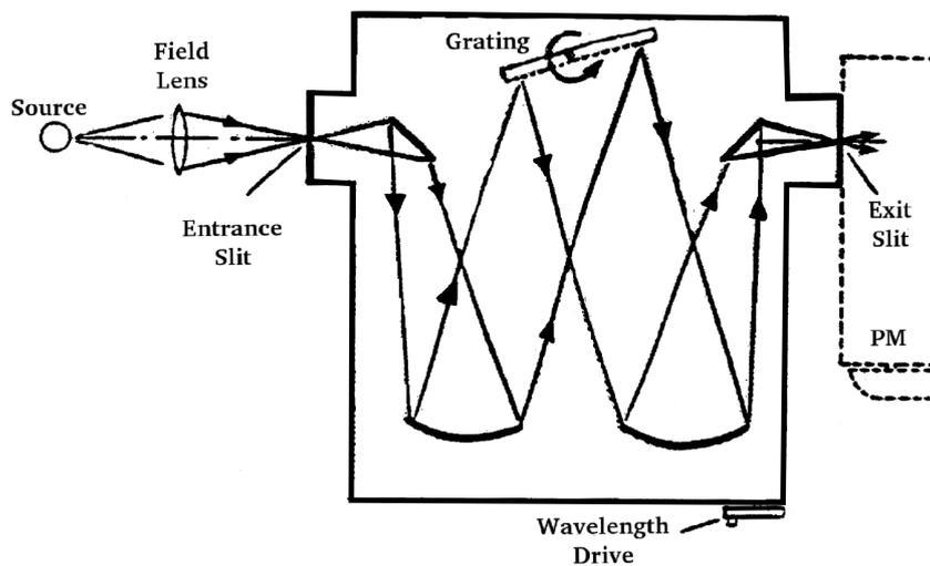
Figure 1.1: The Czerny-Turner Monochromator (the field lens is optional).
