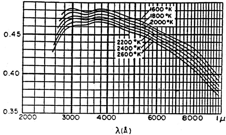
Figure 1.4: Emissivity curves of Tungsten (Devos, Physics 20, 690, in reading room. See the class website for an updated, electronic version)
