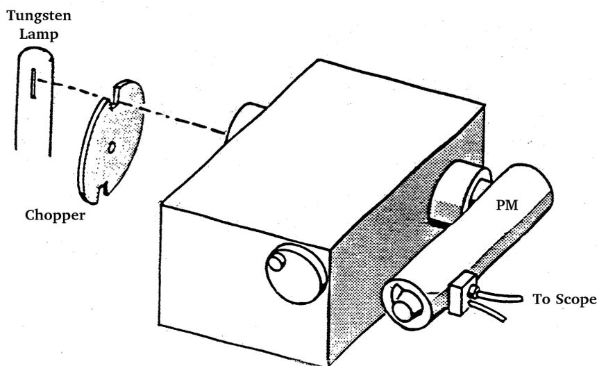
Figure 1.5: Experimental arrangement for measuring the wavelength response
