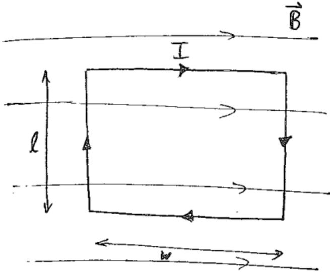
A rectangular loop of wire with width  $w$  and height  $l$  sits in a constant magnetic field that points to the right. The wire will
