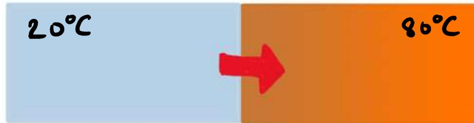
A flow of heat from a cold object to a hot object (without any associated work) would violate conservation of energy.
