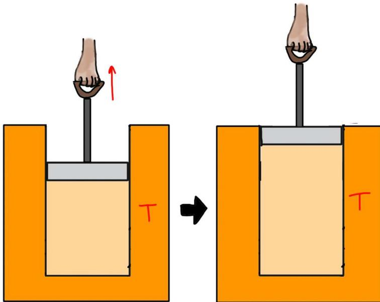
Gas in a cylinder is slowly expanded while in contact with a heat reservoir so that its temperature remains constant. During this process, we can say that
