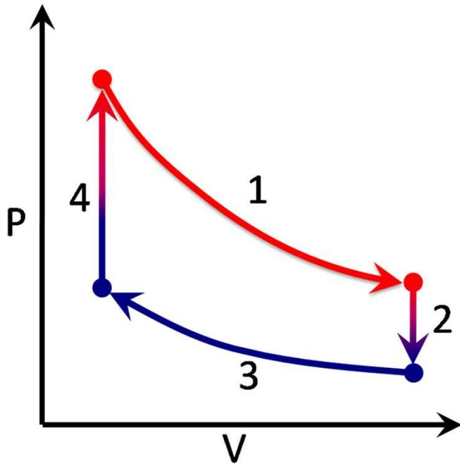
In the process 4, the pressure increases from 100kPa to 250kPa. If the initial temperature is 400K, the final temperature is
