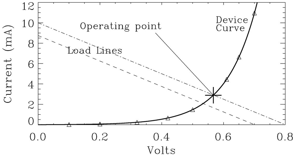
Figure 1: The characteristic curve for a diode is shown as (simulated) data points with a smooth curve passing through them. The dot-dashed line is a load-line for 0.8 volts applied across the device and an  $80\Omega$  resistor connected in series. The dashed line is a similar load line for 0.7 volts.
