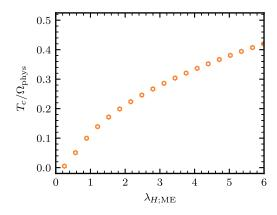
FIG. 15. Transition temperature  $T_c$  in Migdal-Eliashberg theory calculations of the Holstein model divided by the physical (renormalized) phonon frequency  $\Omega_{\rm phys}$  calculated as a function of the conventional Migdal-Eliashberg coupling constant  $\lambda_{H:\rm ME}$  from Eq. (E16).
