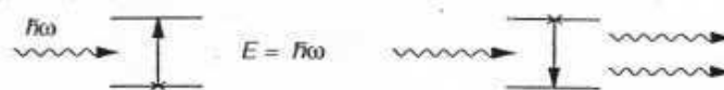
(b) Resonant interaction of photons or phonons with two-level systems. Absorption (left) and induced emission (right) of a photon or phonon with energy h\nu
