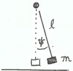
$$\tan \psi = \left| \frac{g'}{g''} \right| = \frac{\omega^2 R_\odot \sin \theta \cos \theta}{g(1 - \omega^2 R_\odot \sin^2 \theta)} \quad (27)$$
