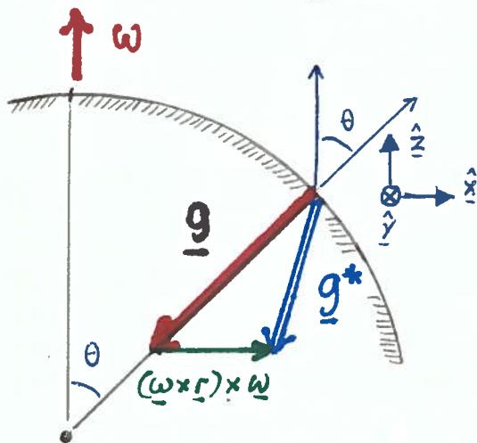
(i) There is a force  $mg$ , acting on a mass  $m$ , from - the earth's gravity - this is directed towards the centre of the earth.
