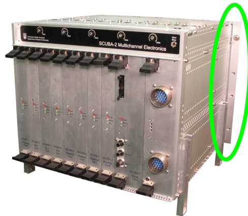
Figure 3.1 Fully-populated subrack with mounting holes highlighted.
