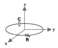
A conducting wire, placed in a magnetic field  $\vec{B} = B_0 \sin(\omega t)\hat{z}$ , forms a circular loop and lies in the z = 0 plane with a radius of 0.1 m. The magnitude of the field is  $B_0 = 0.2$  Tesla, and  $\omega = 10^3$  rad/s. The wire is connected in series to a 5  $\Omega$  resistor and a 100  $\mu$ F capacitor, as shown. Determine the current in the conducting wire. Justify any approximations you make.
