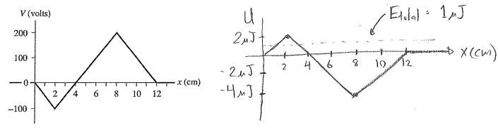
Suppose this charged particle is shot from the right (at x > 12 cm) with a kinetic energy of 1 microjoule.
