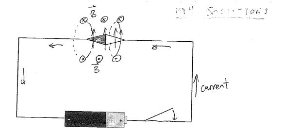
Question 1: In the picture, a compass needle sits directly above a wire that passes 1cm below it (we are looking down from the top). When the switch is closed,
