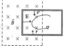
The current inside the magnetic field experiences a force. The top and doflows forces cancel. The force of the left side of the loop makes the loop shoot out to the right
