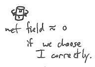
a current loop has a mag. field like a permanent magnet. Thus, if we add a current loop with a field similar to a magnet of the opposite orientation we can nearly cancel the field.
