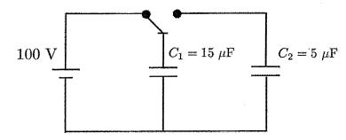
The trick is to realize that the charge is conserved and spread over both capacitors. What is the voltage across each capacitor after the switch is flipped?
