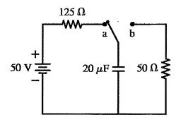
a) Plot the potential across the capacitor as a function of time. What does the plot of the voltage across the resistor look like?
