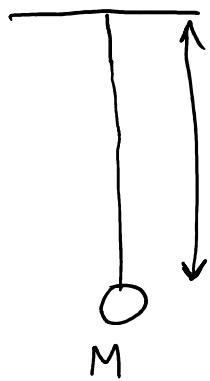
The tension in the string will be  $Mg$ , so the wave speed on the string is
