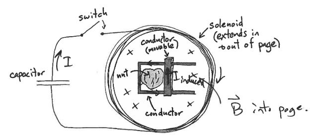
**Question 11:** Back at Sally's So-So Inventions, Sally has just come up with an idea for a not-entirely-practical electromagnetic nut cracker, depicted above. To crack a nut, Sally closes the switch, which discharges the capacitor through a solenoid. When the capacitor is discharged, a movable conductor inside the coil is observed to slide forcefully along another conductor, cracking the nut.
