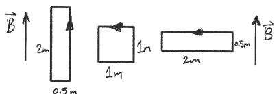
Question 6: The three rectangular current loops shown have equal current and are in equal magnetic fields. Which experiences the greatest torque?
