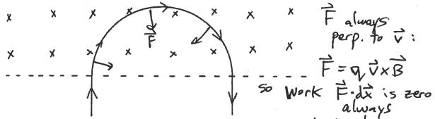
Question 4: A charged particle enters a magnetic field, follows a circular path, and exits the magnetic field again. Assuming there are only magnetic forces on the particle, we can say that the speed of the particle when it exits the field will be speed.
