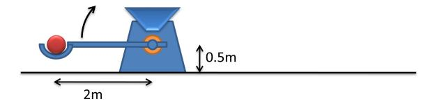
**Question 28:** A 100kg iron ball is loaded into a catapult that starts off in the position shown. When it is fired, the catapult exerts a torque on the lever arm that increases linearly with time:
