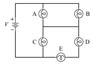
**Question 10:** If all the lightbulbs in the circuit above have equal resistance, which is brightest?
