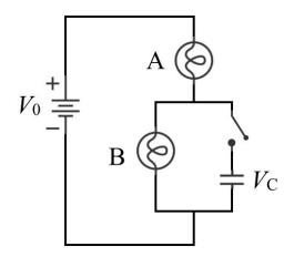
**Question 11:** The switch in the circuit above is closed for a long time. When the switch is opened, what best describes what happens in the circuit above?
