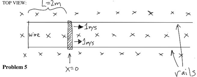
Two perfectly conducting rails separated by 1m sit in a uniform downward magnetic field of 1T. The rails are connected at one end by a fixed perfectly conducting wire, and a freely movable bar with mass 1kg and resistance 1 Ohm is placed across the rail with an initial velocity of 1m/s away from the end.
