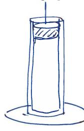
The cylinder is insulated, so we have an adiabatic process with Q=0 and  $\Delta E=N$ . We have  $\Delta E=n\cdot C_V\Delta T$  and  $W=F\Delta x$ , so the required force is given by
