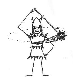
The forces on the ball are gravity and the tension in the chain. Since acceleration is toward the center of the circle for circular motion, the net force must be in this direction.
