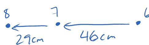
$$\frac{\Delta x_{68}}{\Delta t_{68}} = \frac{-(29\text{cm} + 46\text{cm})}{2 \times 0.545\text{s}}$$
