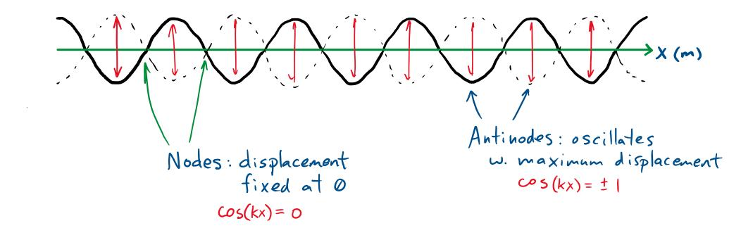
Example : guitar/violin string - displacement must be zero at ends Q: What are the possible wavelengths. for standing waves on a guitar string w. length 1m?
