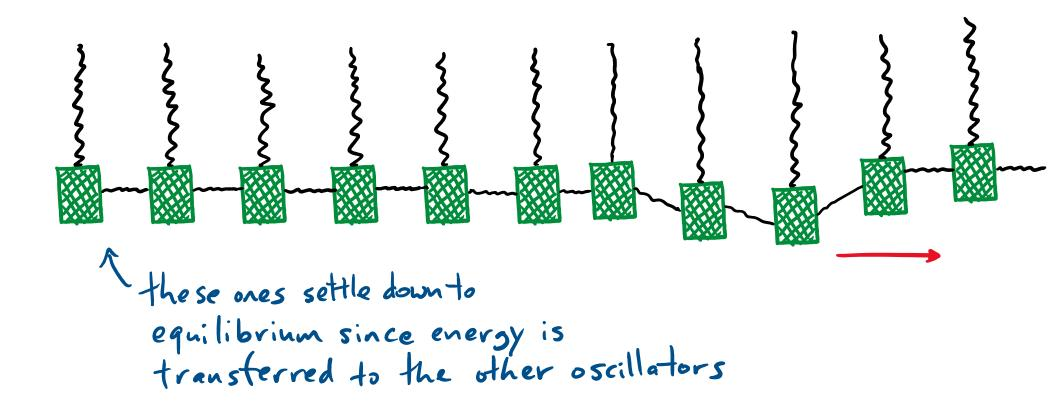
Coupled oscillators: if we drive the leftmost oscillator...
