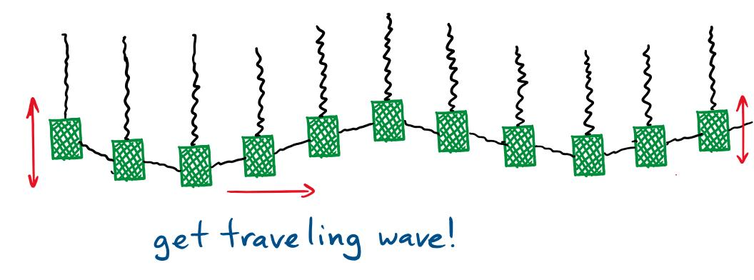
Transverse wave: oscillations perpendicular to direction wave travels
