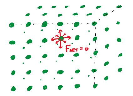
Solid: each atom is in an equilibrium position - displaced atoms feel restoring force
