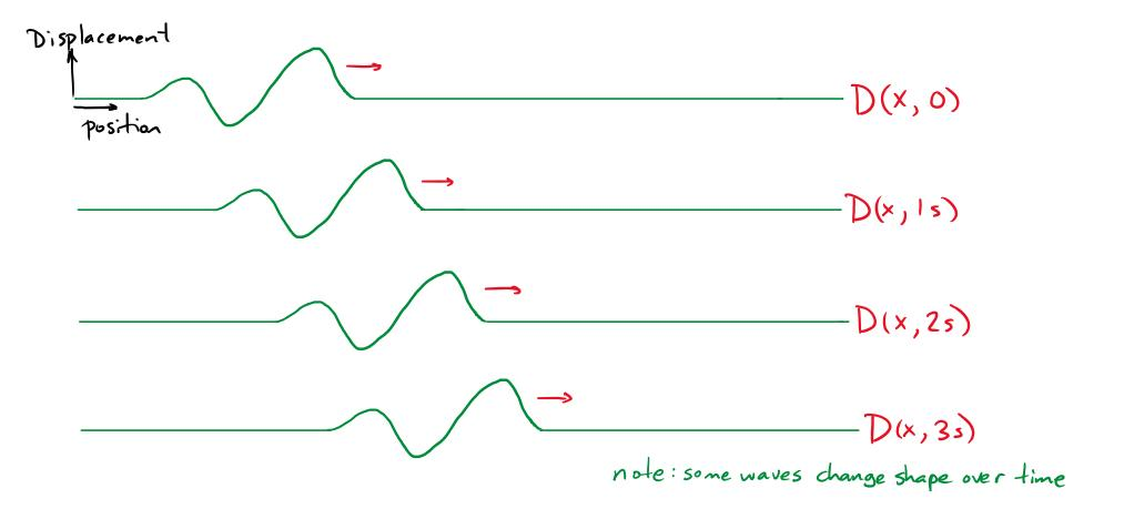
The graph to the right shows D(x, 0), the snapshot of a right-moving wave pulse at time t=0. Which of the graphs below could represent D(2cm,t)?
