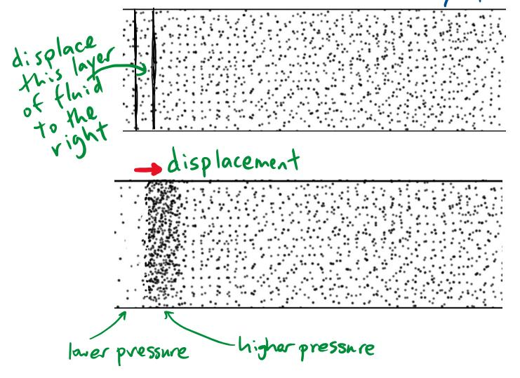
Sound in a fluid : longitudinal waves
