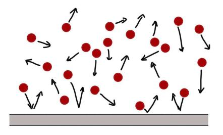
The picture shows molecules of an ideal gas near the wall of a container. What properties of these molecules does the pressure on the wall (force per unit area) depend on?
