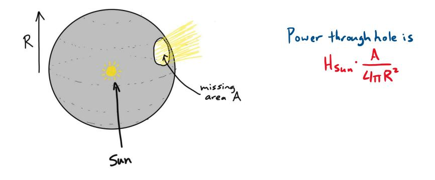
INTENSITY of sunlight (power per area) is  $I = \frac{H_{sun}}{4\pi R^2} \rightarrow \text{double } R \Rightarrow \frac{1}{4} I$ At distance of Earth,  $I = I_{sc} = 1367 \text{ W/m^2}$
