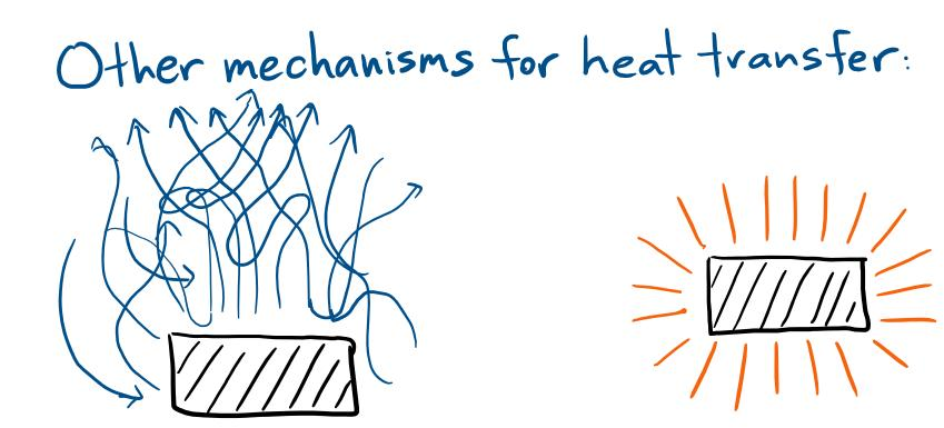
CONVECTION: heat transfer via macroscopic motion of fluids
