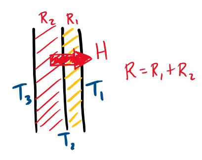
How to show this:  $T_3 - T_2 = \frac{H}{A} \cdot R_2$  $T_2 - T_1 = \frac{H}{A} \cdot R_1$ Add Mese:  $T_3 - T_1 = \frac{H}{A}(R_1 + R_2)$ het temp. A A difference current difference
