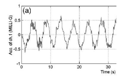
Fig.1. Shows the recording of an accelerometer placed at the height of 298.34 m of the building Di Wang Tower located in Shenzhen, China. This recording of data was taken during a strong wind. Vertical scale is in MILLI-G which is 1/1000 of g (g is the acceleration due to gravity so 1 MILLI-G =  $9.8 \times 10^{-3} m/s^2$ ).
