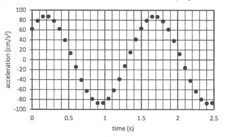
Problem 3. A plot of the acceleration as a function of time for a mass on a spring is shown.
