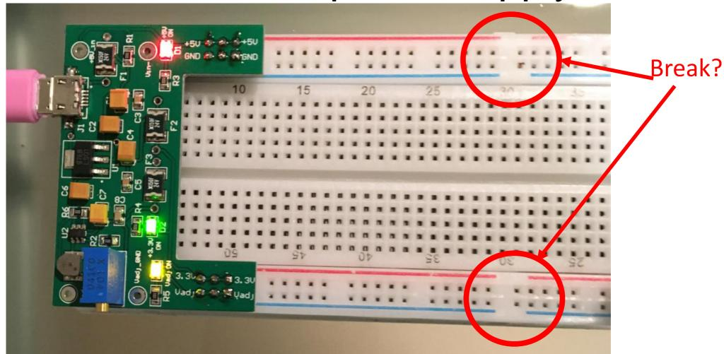
Notice 5V and 3.3V power supply, different than for 219 Adjustable voltage on the power supply (Vadj): Do not use it to power anything! It is only a low current reference voltage and it does not go to 0.
