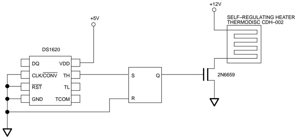
**FAN CONTROL WITH EXTERNAL LATCH** Figure 4
