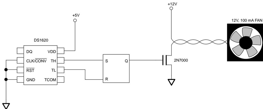
**USING THE T<sub>COM</sub> OUTPUT TO DRIVE A FAN** Figure 5
