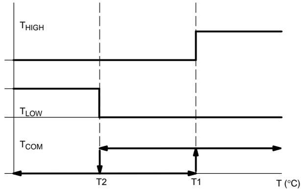
**USING  $T_{HIGH}$  TO DRIVE A FAN** Figure 2
